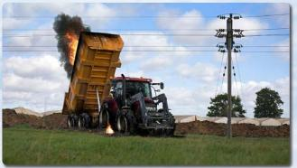
immediately and remain inside the vehicle until the power line is de-energized. In case of smoke or fire, exit the cab by making a solid jump out of the cab (without touching it), and hop away to safety.
